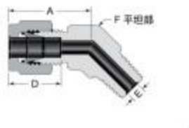
Elbow Pipe Butt Weld 23
